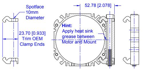
Note: The excess number of mounting holes are so the motor can be raised when the 1 inch spacer block is used between the headstock and base.
